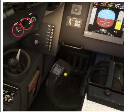
Two Light-Switches, the same Switches are on the Copilotside too
