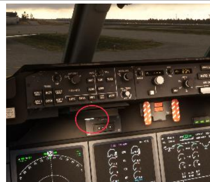
Display Panel Light ON dimnable / the Light is locatet on the ceiling of the cabin
