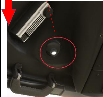
Maplight is located on the ceiling of the cabin
